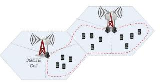
Co-locate A8-Ein (ac) with existing 3G/LTE cell site to offload traffic for an almost identical cell area.
