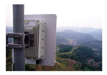
The A8-Ein (ac) is a multi-radio base station utilizing 8x8 MIMO smart antenna technologies and a patented signal processing algorithm to provide the industry's best coverage per base station, especially in non-line-of sight (NLOS) environments. The multi-beam antenna array of the A8-Ein (ac) is designed to provide up to 5 times the range and 10 times the per site coverage as standard access point. Accordingly, up to 90% fewer installation sites for the same coverage area.
