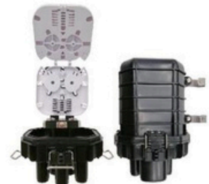
Size: 147.3 \times 104 \times 207.6 \text{mm} PP Material, 48 fibers 3 round ports + 1 oval port Heat shrinkable sealing
