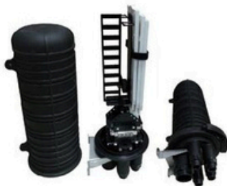
Size: \Phi 146 \times 300.5 mm PP Material 48 fibers 3 round & 1 oval port, Heat shrinkable sealing
