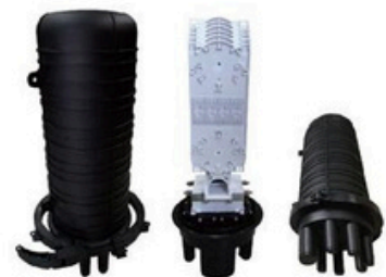
Size: \Phi 168 \times 434.5 mm PP Material 120 fibers 3 round & 1 oval port, Heat shrinkable sealing
