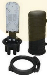
Size: \Phi 146 \times 310.5 mm PP Material 48 fibers 4 round Port, Mechanical sealing
