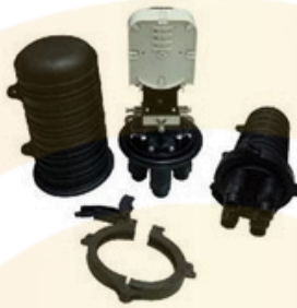
Size: \Phi 139.8 \times 349.1 mm PP Material 48 fibers 1 oval & 4 round port, Heat shrinkable sealing
