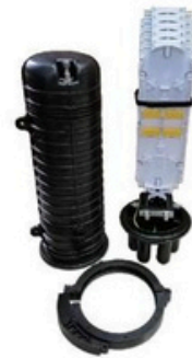
Size: \Phi 204.2 \times 549 \text{mm} PP Material 144 fibers 4 round & 1 oval port, Heat shrinkable sealing
