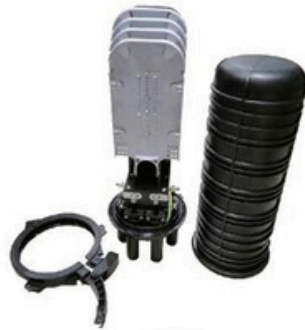
Size: \Phi 182.5 \times 509.1 \text{mm} ABS+PC Material 576 fibers 4 round & 1 oval port, Heat shrinkable sealing
